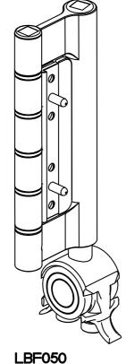
Double Roller Top/Btm Note: Top Roller Sprung Loaded
