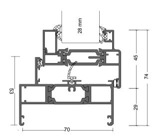
This shows the Stepped sash in the AW605 frame, which is an equal leg frame but 10mm deeper than the AW604.
