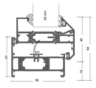
This shows the Feature sash in the AW605 frame, which is an equal leg frame but 10mm deeper than the AW604.
