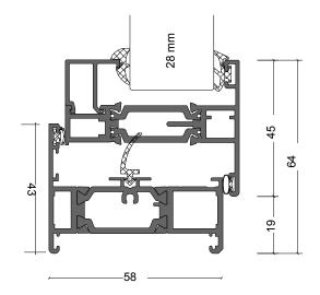
This shows the Flat sash in the AW605 frame, which is an equal leg frame but 10mm deeper than the AW604.
