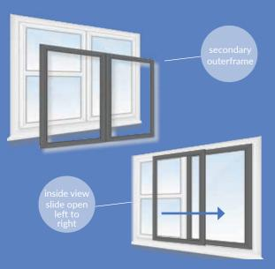
By selecting the right design (see opposite) for the right place, your secondary glazing will improve any primary window that it is fitted to, whilst being sympathetic on the eye.
