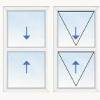
Hinged: Opening inwards, hinged units provide full access to the primary window. Single or double openers are available for both domestic and commercial sized windows. Hinged units are perfect for fire escapes and for French or Patio doors.
